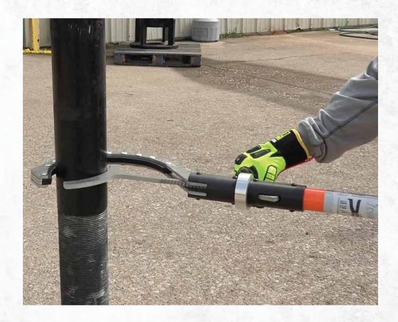
Grasp and manipulate tubular or cylindrical objects ranging from 3 to 10 inches in diameter.
