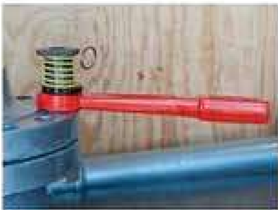
Place wrench on nut and thread retainer onto stud.
